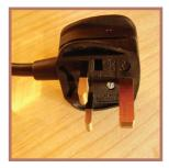
The Plugs and Sockets etc (Safety) Regulations 1994 require all electrical appliances, both new and existing, to be fitted with an approved plug with sleeved pins when supplied to a consumer. All plugs should carry the name and reference number of the approved body (e.g. BSI). All sockets (e.g. on mains extension leads), adaptors and similar devices must meet British or European Standards.
