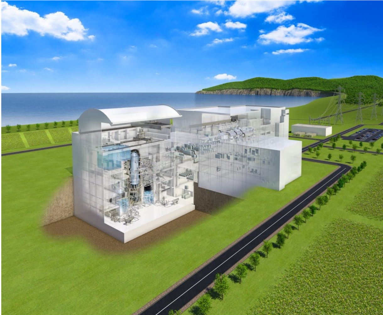
Figure 5.4 Schematic of UK ABWR
