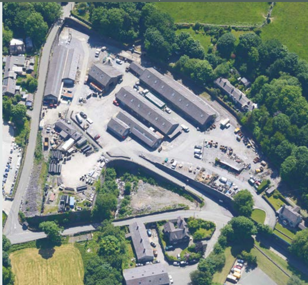
The Felin Fawr complex of industrial buildings in the Ogwen valley (Component Part 1) served Penrhyn quarry until the 1960s. Here slabs were sawn. Waterwheels powered by the Galedffrwd stream turned the machinery © Crown copyright: RCAHMW.
